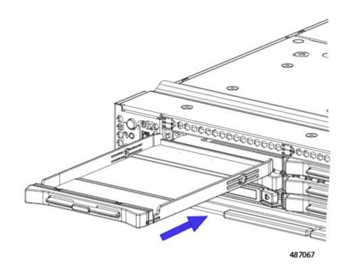
Installing a Drive Blank Filler
