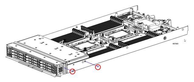
**Step 6** Replace the compute node top cover and reinstall the compute node into the chassis. See Installing a Compute Node Cover, on page 6.
