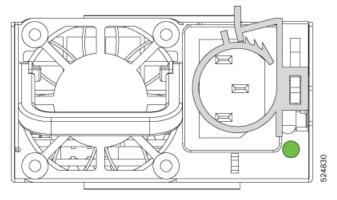
Replace a power supply with another supported power supply that has the same power source type as the other installed power supply. Additionally, the airflow direction of the power supply must match or conform to the airflow direction of the installed fan modules.
