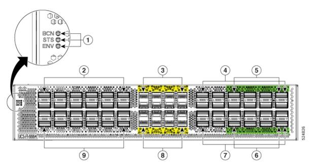
The following table shows the contents of the fabric interconnect front panel. Ports are arranged in vertical columns as two pairs of ports.
