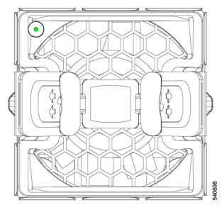
Each fan module has a Status LED that indicates the health of the fan module.
