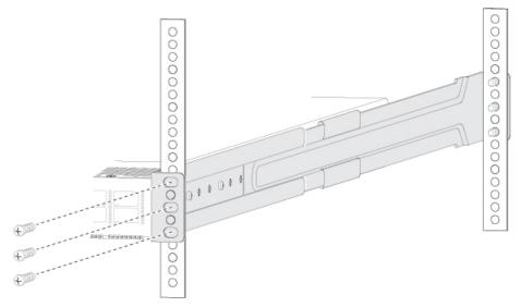
d) Tighten the 10-32 screws to 20 in-lb (2.26 N·m) or tighten the 12-24 screws to 30 in-lb (3.39 N·m).
