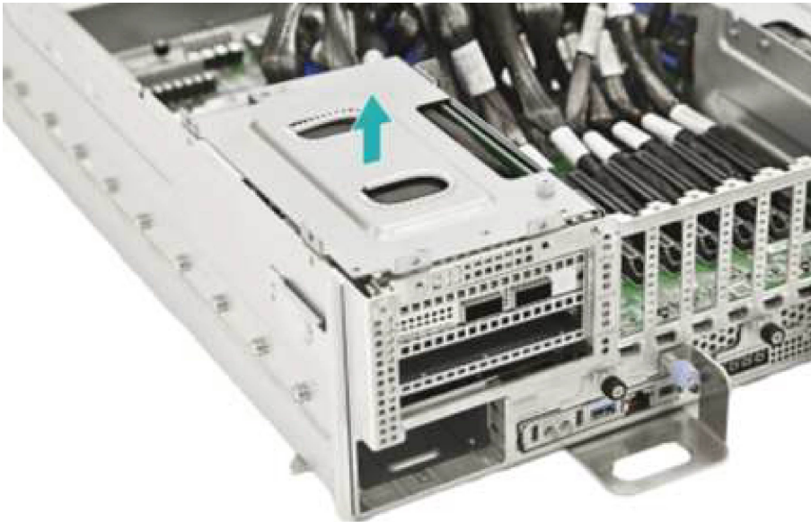
Figure 7: Removing the CEM Riser Assembly (Right CEM)
