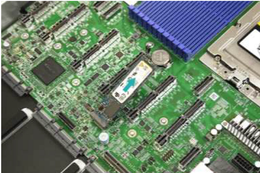
Figure 20: Removing the SSD from the Mainboard
