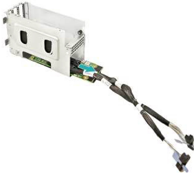
Figure 10: Removing the CEM Riser
