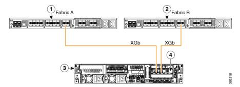
Cisco IMC on the C-Series Rack-Mount Server uses the first adapter for management and data connectivity and a second adapter only for data connectivity. Every virtual interface on the rack server needs to be connected to both Fabric Interconnect adapters. Different configurations require specific setup. For detailed instructions, use the information provided in the section *Physical Connectivity Illustrations for Direct Connect Mode Cluster Setup* in the appropriate C-Series Integration Guide.
