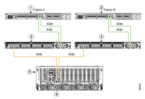
Figure 4: SingleConnect Cabling Configuration with Cisco VIC 1455/VIC 1457/VIC 1467/VIC 15428
