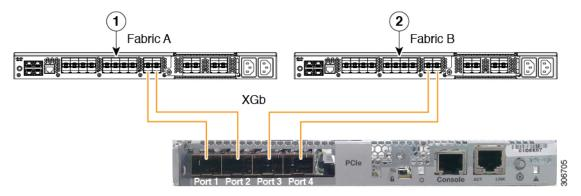
Figure 11: Direct Connect Cabling Configuration with Cisco VIC 1455 (2-Port Linking)
