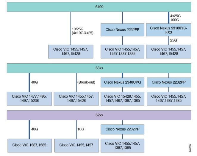
Figure 2: Network Topology for 6200, 6300, and 6400 Series Fabric Interconnect with 1300/1400/15000 Series VIC Cards
