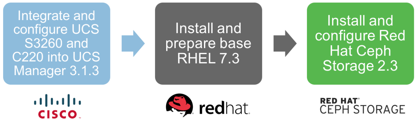
Figure 9 Deployment Parts for Red Hat Ceph Storage on Cisco UCS
