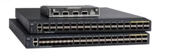
The Cisco UCS 6300 Series provides the management and communication backbone for the Cisco UCS B-Series Blade Servers, 5100 Series Blade Server Chassis, and C-Series Rack Servers managed by Cisco UCS. All servers attached to the fabric interconnects become part of a single, highly available management domain. In addition, by supporting unified fabric, the Cisco UCS 6300 Series provides both LAN and SAN connectivity for all servers within its domain.
