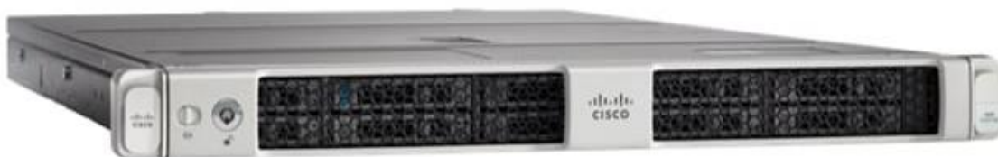
Figure 9. Cisco UCS C220 M7 Rack Server
