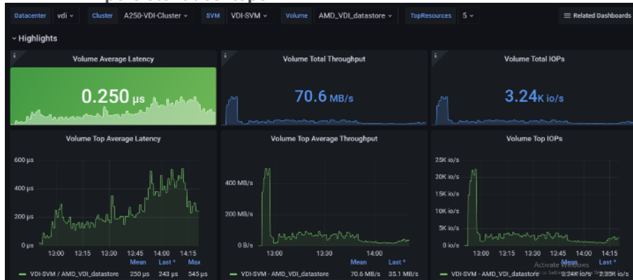
Figure 78. Volume Average Latency, Volume Total Throughput and Volume Total IOPS AFF A250 volume 1 for 500 persistent desktops
