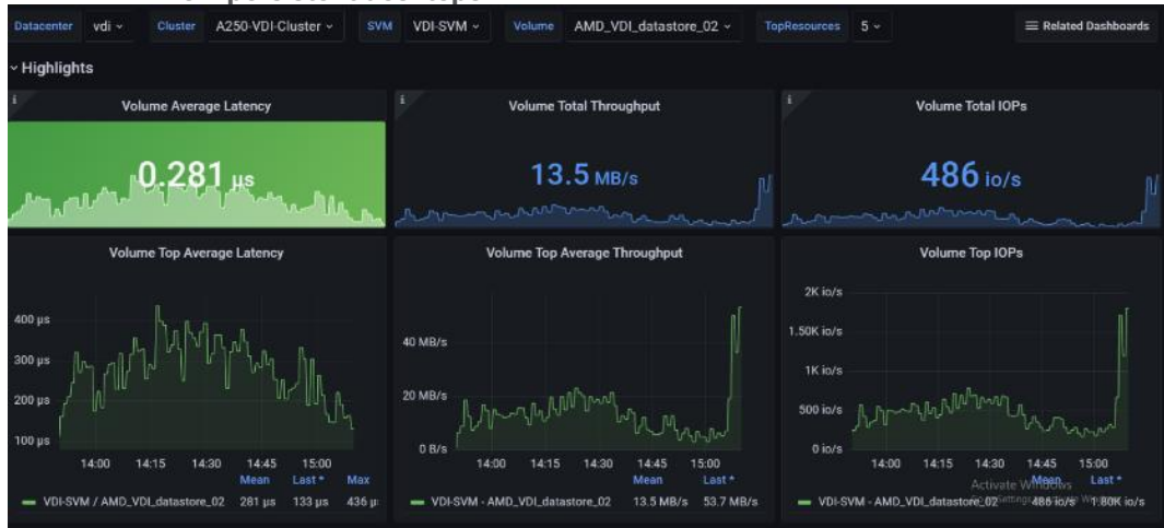
Figure 83. Volume Average Latency, Volume Total Throughput and Volume Total IOPS AFF A250 volume 2 for 500 non-persistent desktops
