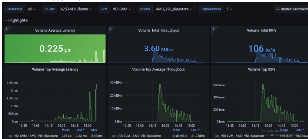
Figure 74. Volume Average Latency, Volume Total Throughput and Volume Total IOPS AFF A250 volume 1 for 1000 RDS
