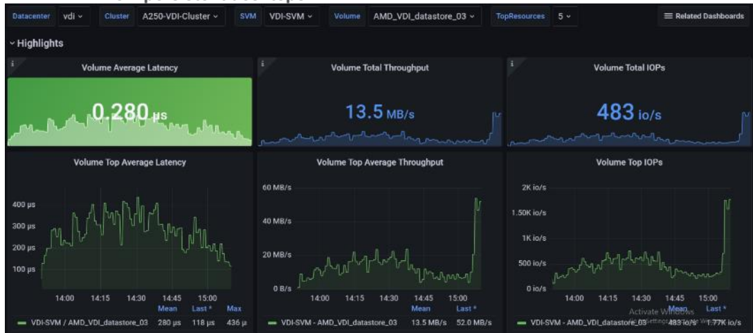
Figure 84. Volume Average Latency, Volume Total Throughput and Volume Total IOPS AFF A250 volume 3 for 500 non-persistent desktops
