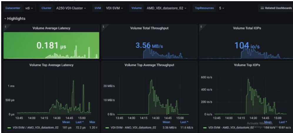
Figure 76. Volume Average Latency, Volume Total Throughput and Volume Total IOPS AFF A250 volume 3 for 1000 RDS
