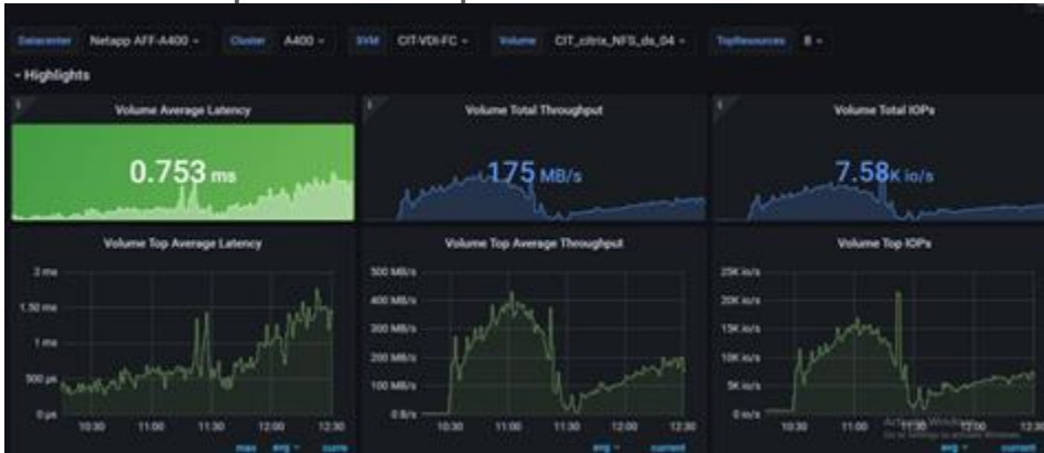
Figure 81. Volume Average Latency, Volume Total Throughput and Volume Total IOPS AFF A400 volume 4 for 2000 persistent desktops
