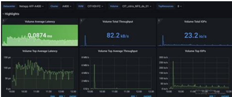
Figure 74. Volume Average Latency, Volume Total Throughput and Volume Total IOPS AFF A400 volume 1 for 2400 RDS
