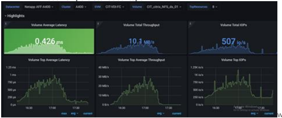
Figure 82. Volume Average Latency, Volume Total Throughput and Volume Total IOPS AFF A400 volume 1 for 2000 non persistent desktops
