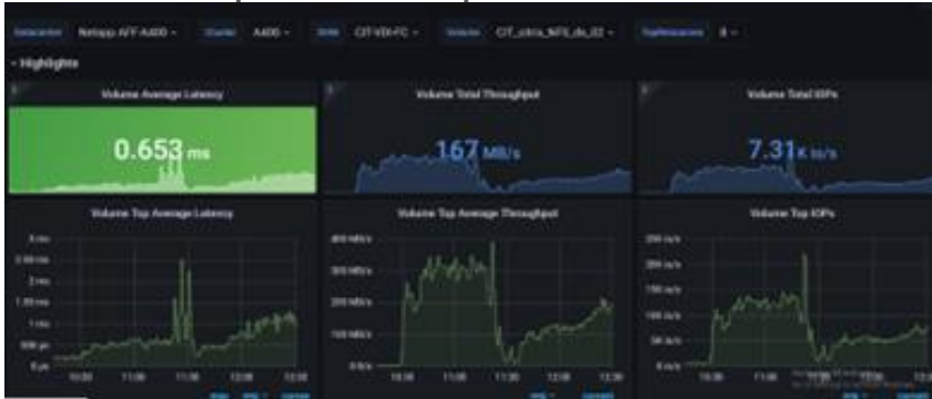
Figure 79. Volume Average Latency, Volume Total Throughput and Volume Total IOPS AFF A400 volume 2 for 2000 persistent desktops
