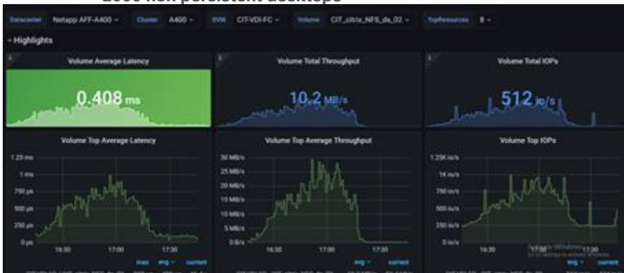
Figure 83. Volume Average Latency, Volume Total Throughput and Volume Total IOPS AFF A400 volume 2 for 2000 non persistent desktops
