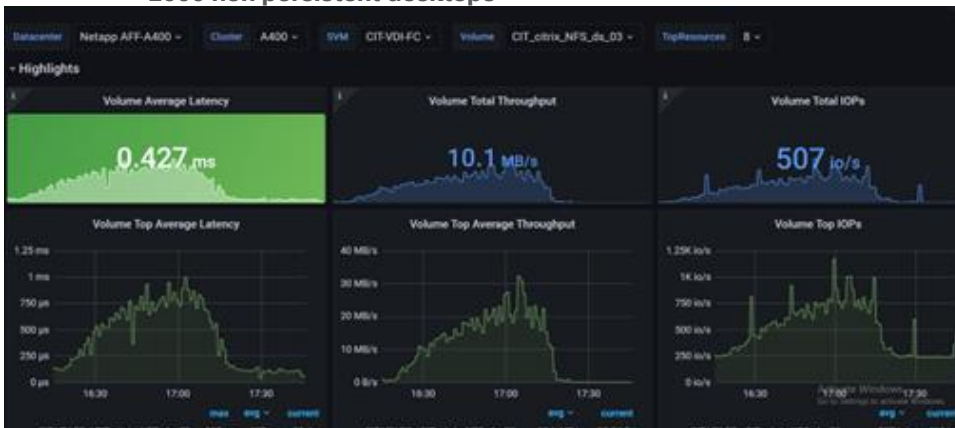
Figure 84. Volume Average Latency, Volume Total Throughput and Volume Total IOPS AFF A400 volume 3 for 2000 non persistent desktops
