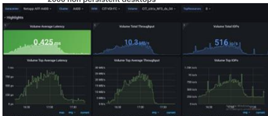
Figure 85. Volume Average Latency, Volume Total Throughput and Volume Total IOPS AFF A400 volume 4 for 2000 non persistent desktops
