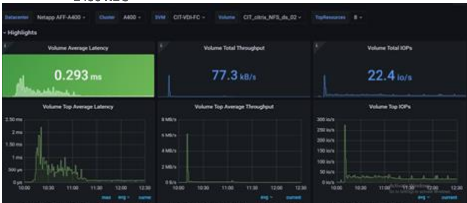
Figure 75. Volume Average Latency, Volume Total Throughput and Volume Total IOPS AFF A400 volume 2 for 2400 RDS
