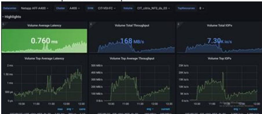
Figure 80. Volume Average Latency, Volume Total Throughput and Volume Total IOPS AFF A400 volume 3 for 2000 persistent desktops
