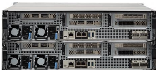
Figure 28. NetApp AFF A800 Rear View
