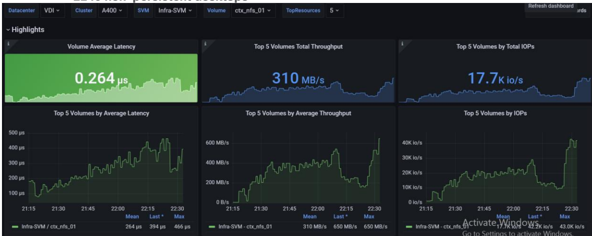
Figure 84. Volume Average Latency, Volume Total Throughput and Volume Total IOPS AFF A400 volume 1 for 2240 non-persistent desktops
