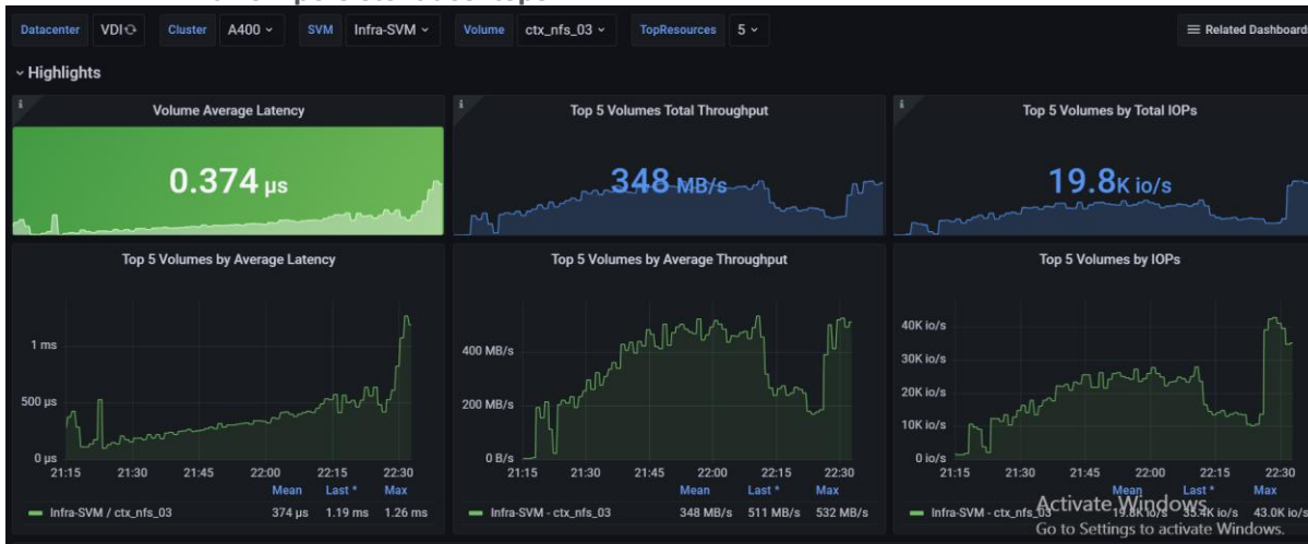
Figure 86. Volume Average Latency, Volume Total Throughput and Volume Total IOPS AFF A400 volume 3 for 2240 non-persistent desktops
