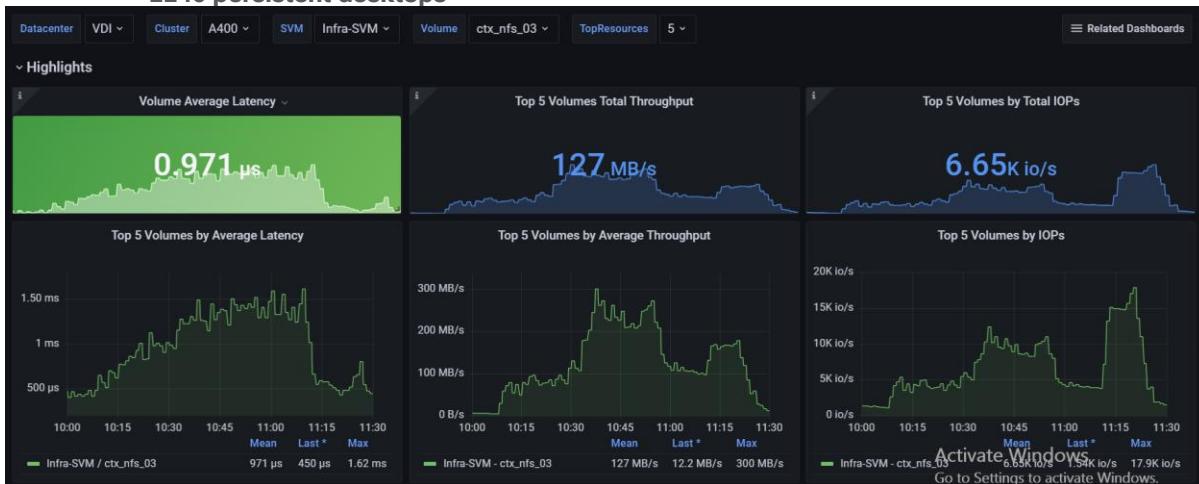
Figure 82. Volume Average Latency, Volume Total Throughput and Volume Total IOPS AFF A400 volume 3 for 2240 persistent desktops
