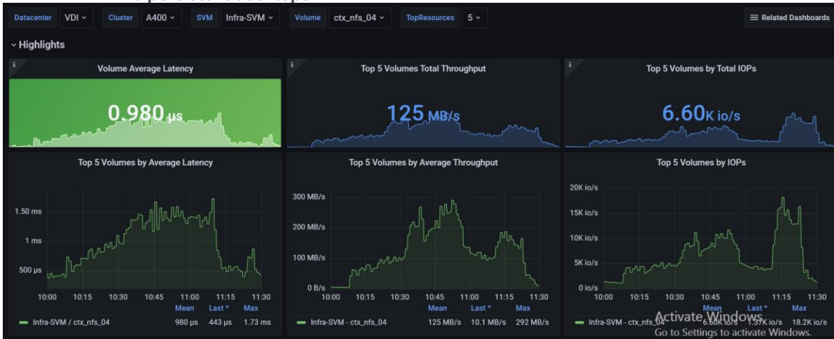
Figure 83. Volume Average Latency, Volume Total Throughput and Volume Total IOPS AFF A400 volume 4 for 2240 persistent desktops
