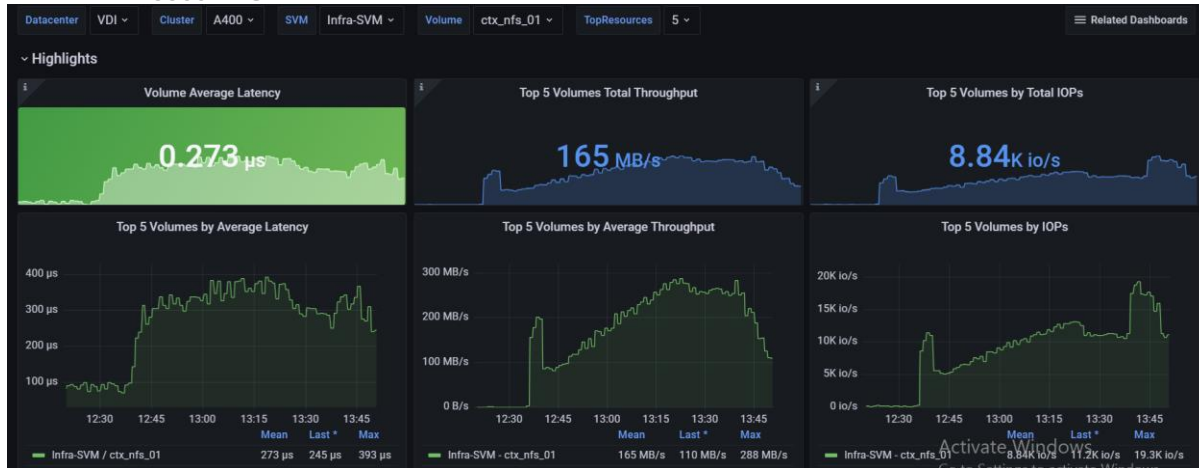
Figure 76. Volume Average Latency, Volume Total Throughput and Volume Total IOPS AFF A400 volume 1 for 3360 RDS
