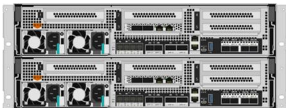
Figure 16. NetApp AFF A400 Rear View
