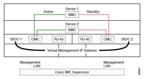
The system uses a chassis management controller (CMC) to manage the server nodes. Each system I/O controller (SIOC) module contains an onboard CMC. If you have two SIOCs, the two CMCs act in an active/standby organization. The CMC in the SIOC that you log into with the Cisco IMC interface becomes the active CMC and it allows you to manage the BMCs in both server nodes.
