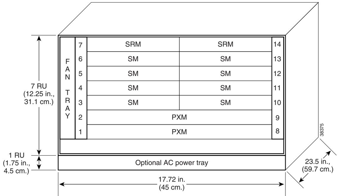
**Figure 1-3 MGX 8230 Card Cage—Font View**
