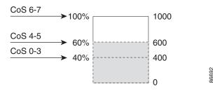
In this example, CoS values 6 and 7 have a greater importance than the other CoS values, and they are assigned to the 100-percent drop threshold (queue-full state). CoS values 4 and 5 are assigned to the 60-percent threshold, and CoS values 0 to 3 are assigned to the 40-percent threshold.
