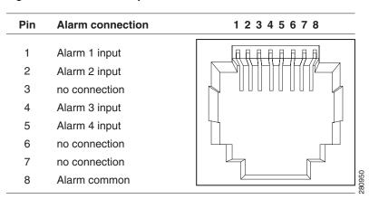
For each alarm input, you can configure an open or closed circuit to trigger an alarm and configure the severity of the alarm. A triggered alarm generates an system message. If you enter a descriptive name for the alarm, that name is included in the system message. A triggered alarm also turns on the LED display (the LED is normally off, meaning no alarm). See the *Cisco ME-3400E Hardware Installation Guide* for information about the LEDs.
