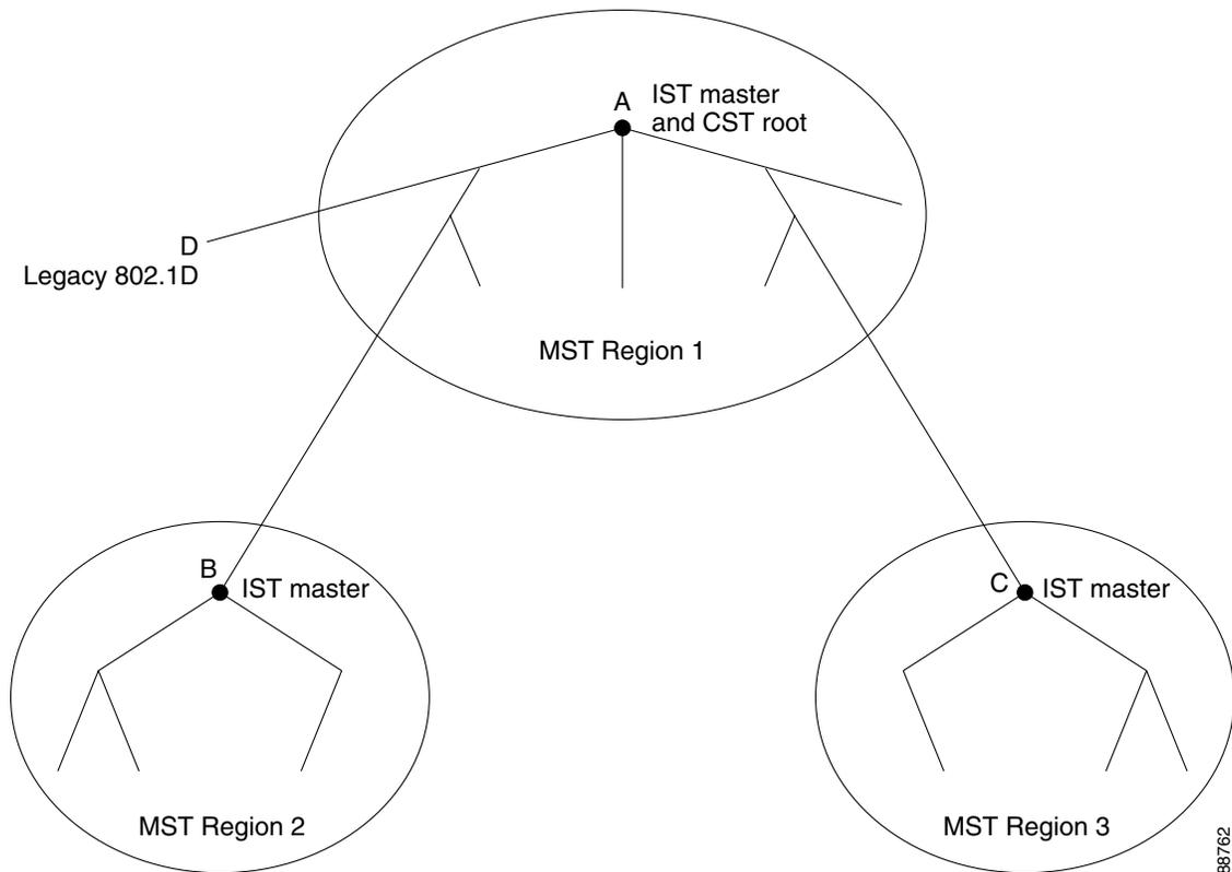
Figure 15-1 does not show additional MST instances for each region. Note that the topology of MST instances can be different from that of the IST for the same region.
