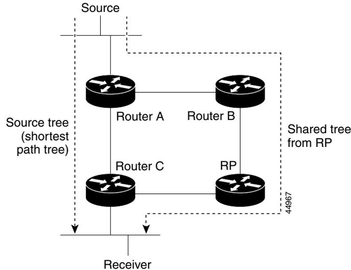
If the data rate warrants, leaf routers (routers without any downstream connections) on the shared tree can use the data distribution tree rooted at the source. This type of distribution tree is called a shortest-path tree or source tree. By default, the software switches to a source tree upon receiving the first data packet from a source.
