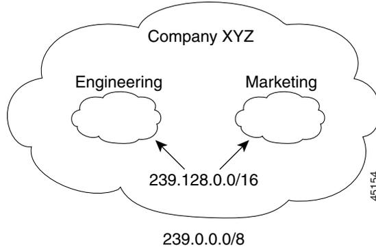
You can define an administratively-scoped boundary on a routed interface for multicast group addresses. A standard access list defines the range of addresses affected. When a boundary is defined, no multicast data packets are allowed to flow across the boundary from either direction. The boundary allows the same multicast group address to be reused in different administrative domains.
