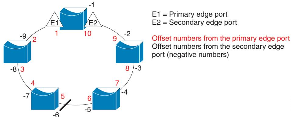
When the REP segment is complete, all VLANs are blocked. When you configure VLAN load balancing, you must also configure triggers in one of two ways:
