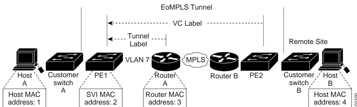
Assume that Host A is connected to the customer switch on VLAN 3 that has a trunk port connected to PE1 configured for 802.1Q tagging. Host A sends a packet to Host B, using the specific values of MAC addresses, labels, and VLANs shown in the figure. The customer switch tags the host packet and forwards it over the trunk port to PE1.
