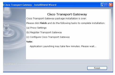
Step 7 When the system detects that the Transport Gateway has not yet been registered on the Cisco backend, the system requests the customer to complete the Transport Gateway installation.
