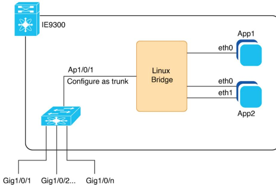
This image depicts the Ethernet and Layer 2 connections within an IOx-enabled network on a Cisco Catalyst IE9300 Rugged Series Switch. The additional interface, Ap1/0/1, is internally connected to a Linux bridge and is configured as a trunk to support multiple IOx applications.
