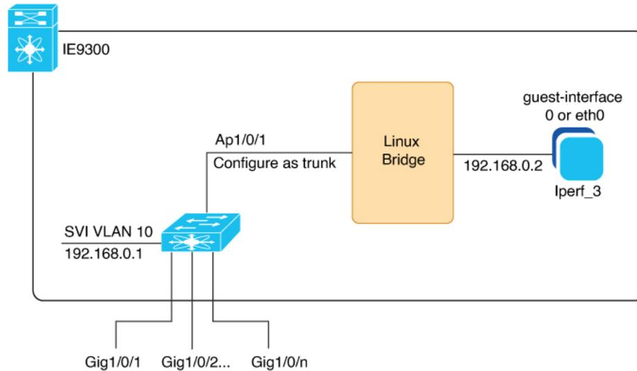
The configuration example here depicts a typical IOx application deployment on a Cisco Catalyst IE9300 Rugged Series Switch. The interface Ap1/0/1 is internally linked to a Linux bridge and set up as a trunk to facilitate multiple IOx applications. The application "Iperf\_3" is assigned the IP address 192.168.0.2 on its guest interface. And the default gateway for the network is configured on the Switch Virtual Interface (SVI) VLAN 10, using the IP address 192.168.0.1.
