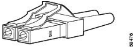
Figure 2: Fiber-Optic SFP Module LC Connector
