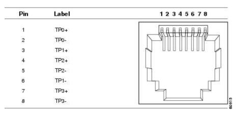
Connector pins 1, 2, 3, and 6 are used for PoE.
