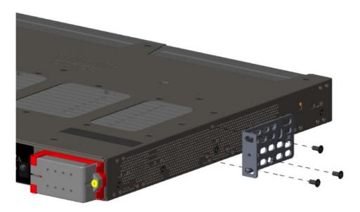
Figure 8: Attaching Brackets for 19-Inch Racks (Rear Mount)
