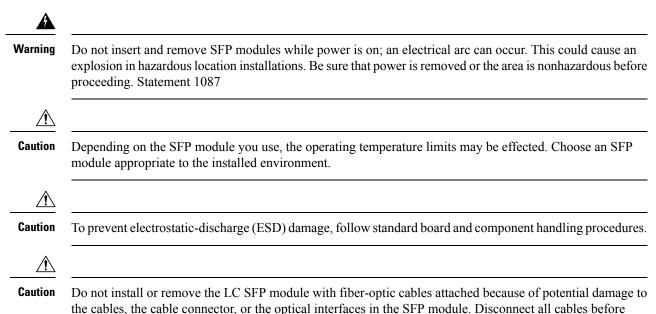
removing or installing an SFP module.
