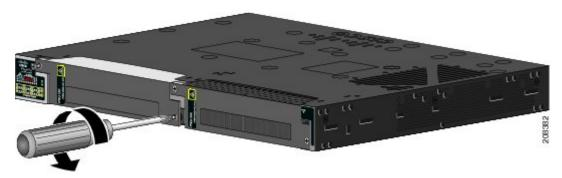
Figure 25: Remove the Power Supply Blank
