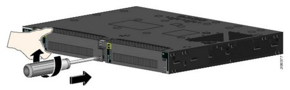
**Step 7** Use a ratcheting torque screwdriver to torque each screw to 8–10 in-lb.
