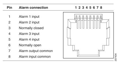
For each alarm input, you can configure an open or closed circuit to trigger an alarm and configure the severity of the alarm. A triggered alarm generates an system message. If you enter a descriptive name for the alarm, that name is included in the system message. A triggered alarm also turns on the LED display (the LED is normally off, meaning no alarm). See the *Cisco Switch Hardware Installation Guide* for information about the LEDs.
