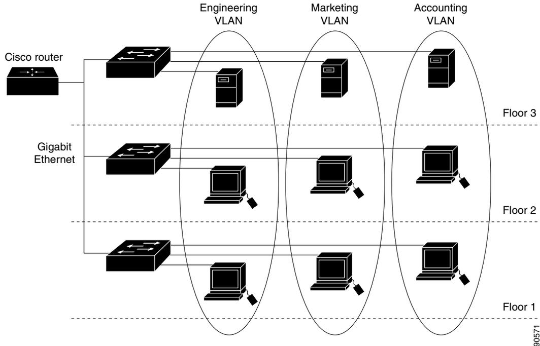
VLANs are often associated with IP subnetworks. For example, all the end stations in a particular IP subnet belong to the same VLAN. Interface VLAN membership on the switch is assigned manually on an interface-by-interface basis. When you assign switch interfaces to VLANs by using this method, it is known as interface-based, or static, VLAN membership.
