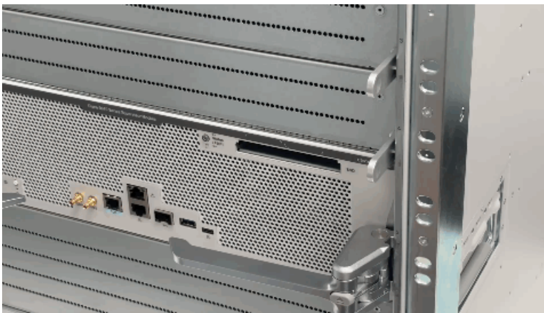
Figure 15: Inserting the SSD module into the slot
