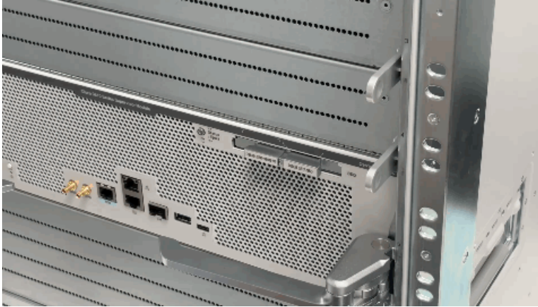
Figure 13: Pressing the release handles
