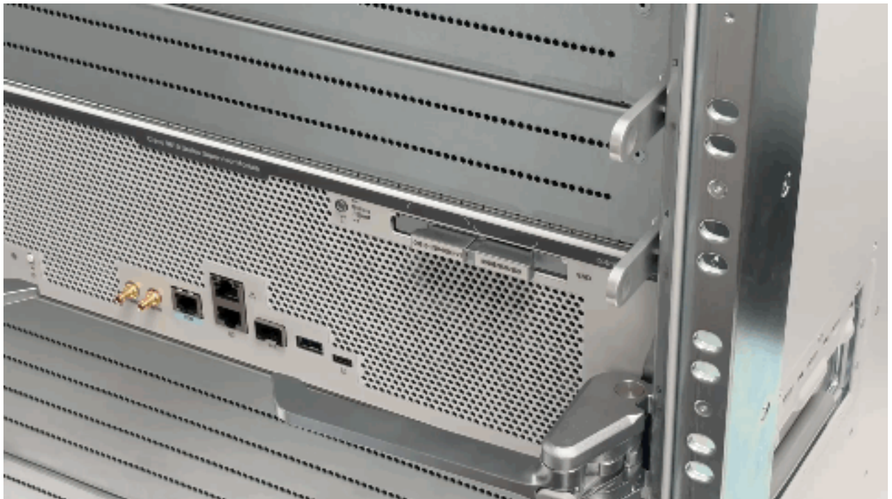
Figure 12: Pressing the SSD status/eject button
