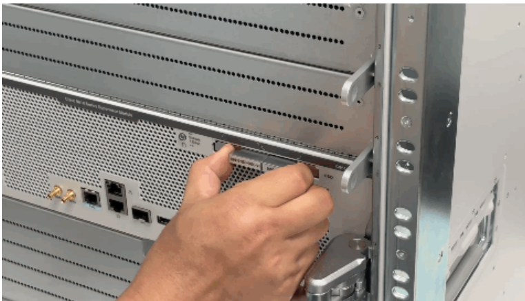
Figure 14: Removing the SSD from the supervisor
