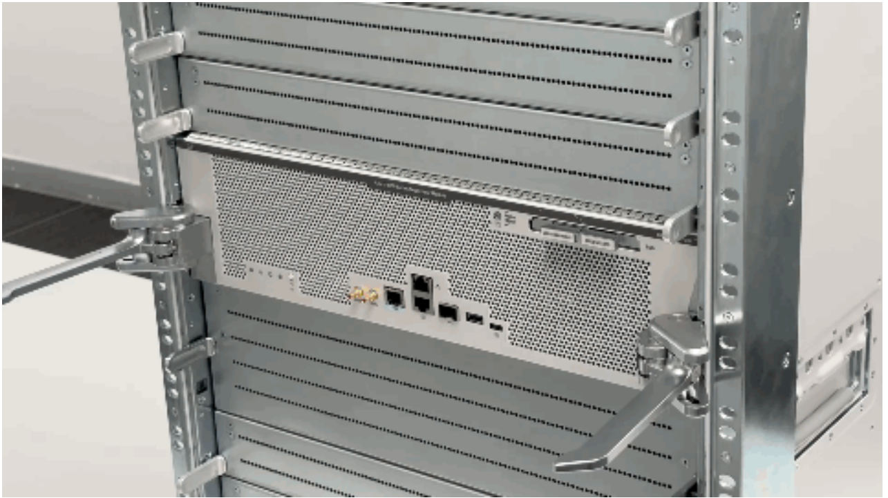
Figure 6: Pulling out the supervisor engine from the slot
