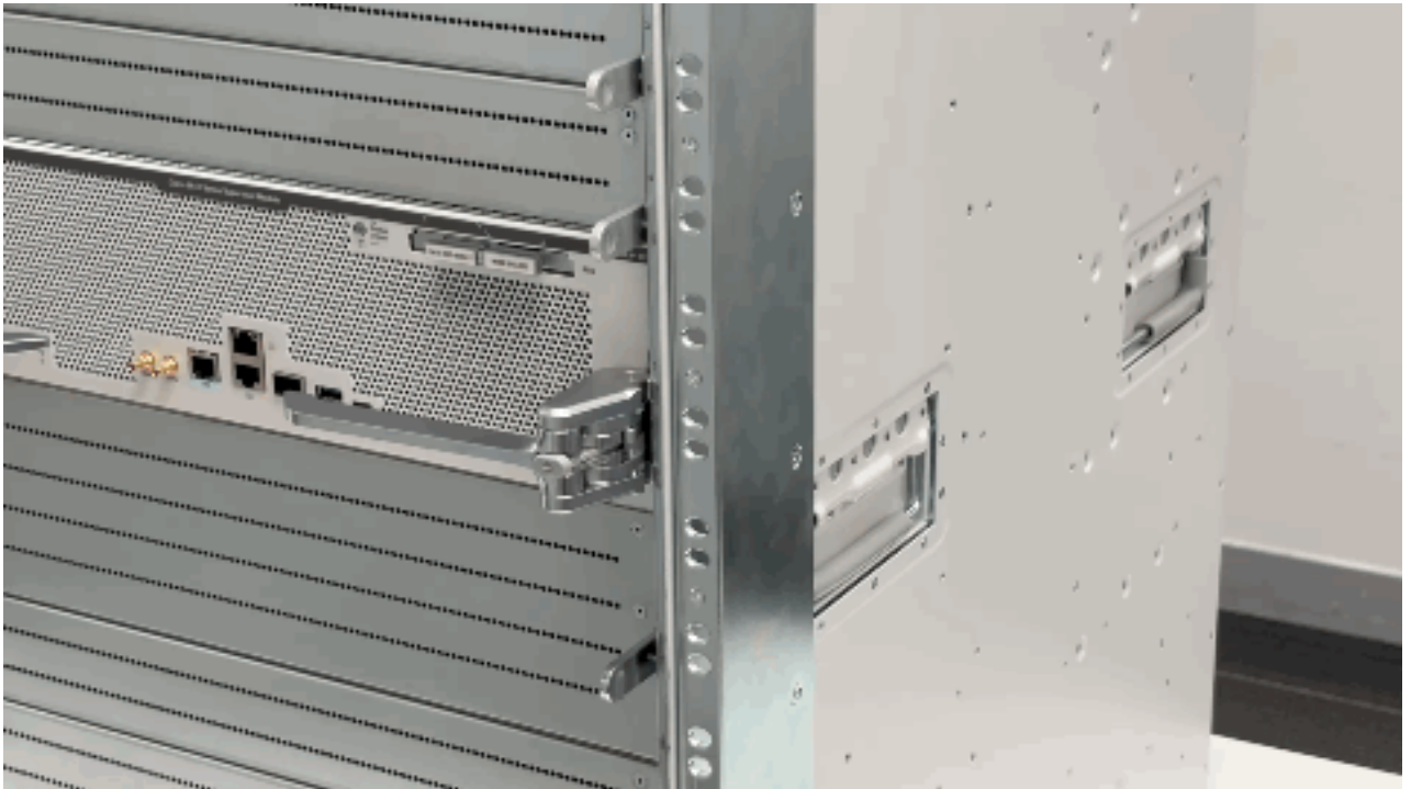
Figure 4: Pressing the ejector lever buttons to unlock the levers
