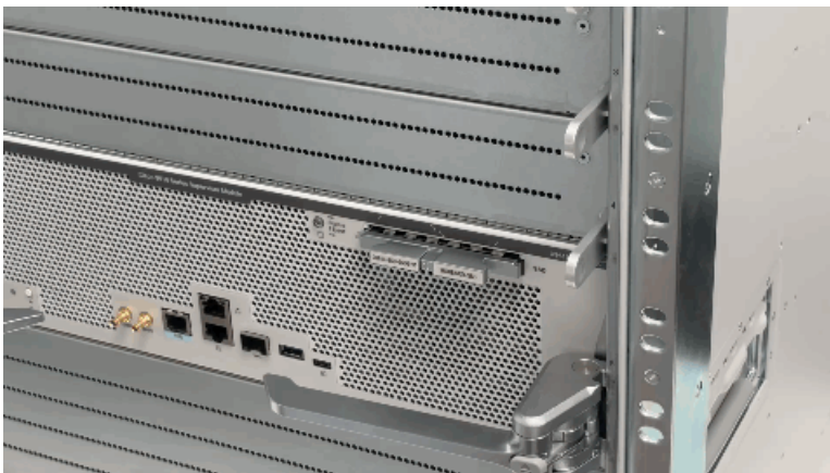
Figure 16: Pressing the SSD module into the connector
