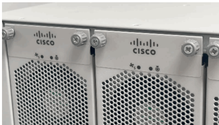
Figure 15: Removing the captive installation screws on the fan tray
