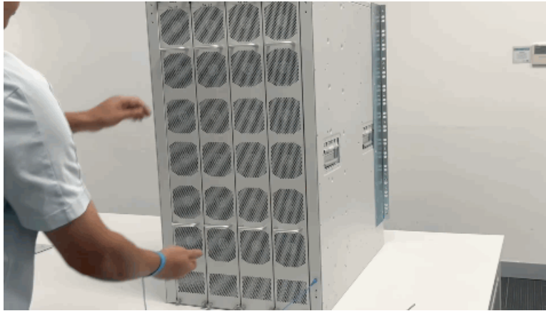
Figure 16: Removing the fan tray assembly
