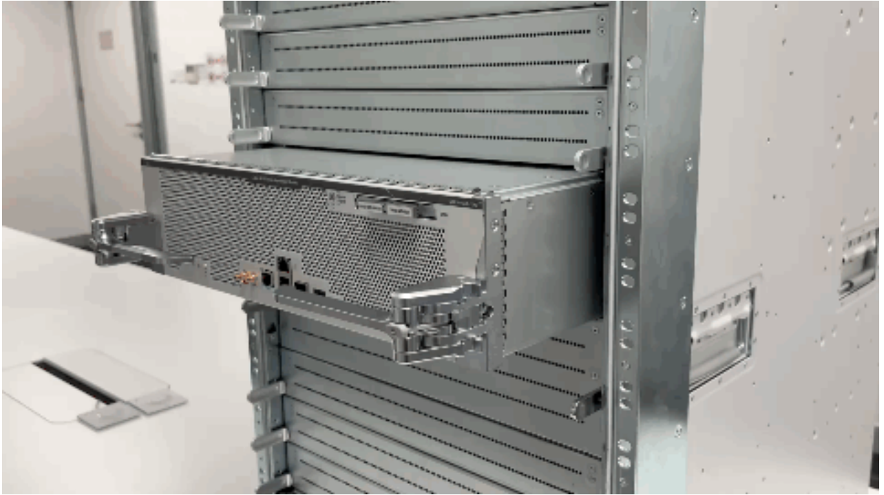
Figure 9: Opening the ejector levers
