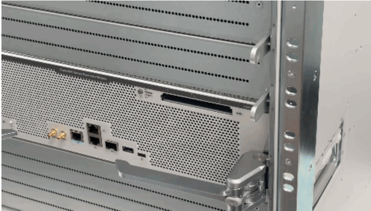
Figure 15: Inserting the SSD module into the slot
