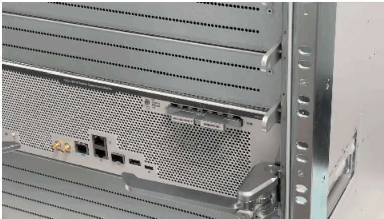
Figure 16: Pressing the SSD module into the connector
