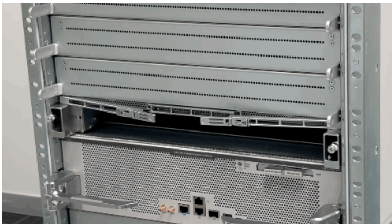
Figure 19: Releasing the ejector lever locks
