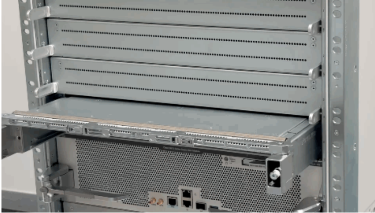
Figure 20: Pulling out the line card adapter
