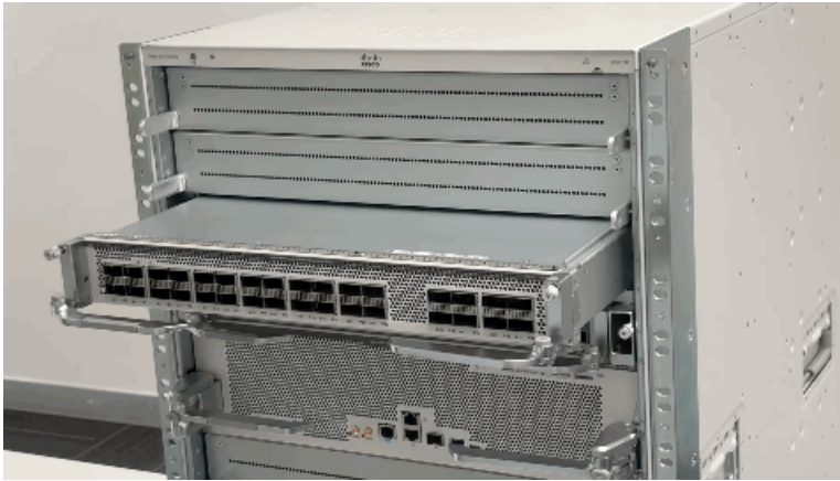
Figure 13: Removing a line card completely from the slot
