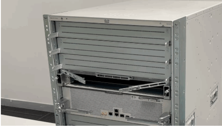
Figure 16: Pivoting ejector levers inward
