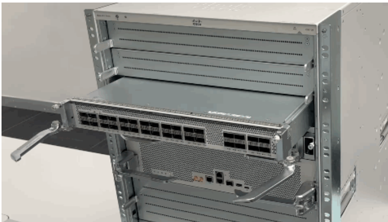
Figure 9: Sliding the line card completely into the slot
