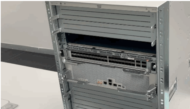
Figure 7: Positioning and sliding the line card into the slot
