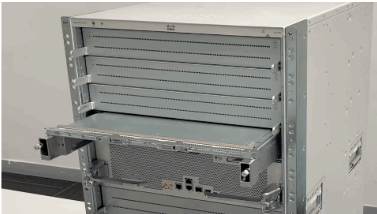
Figure 15: Opening the ejector levers
