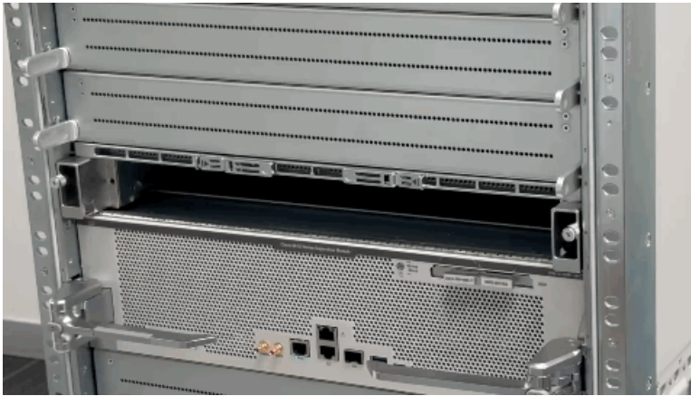
Figure 18: Unscrewing the captive screws
