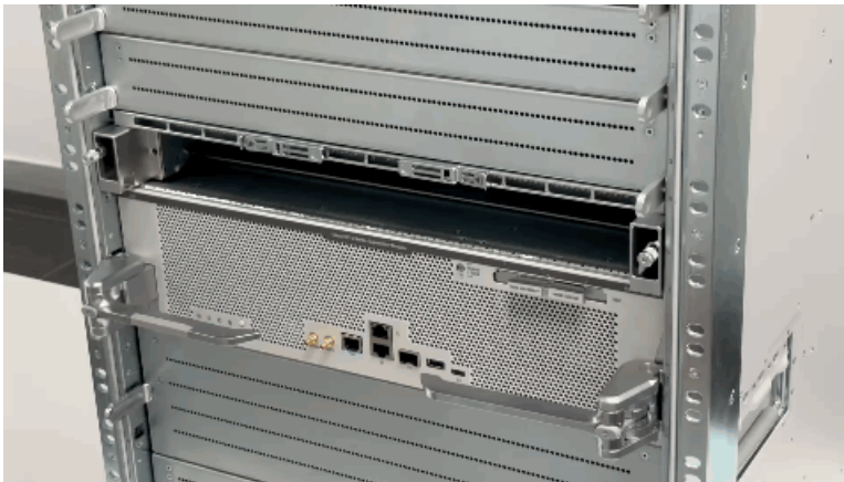
Figure 17: Screwing in the captive screws
