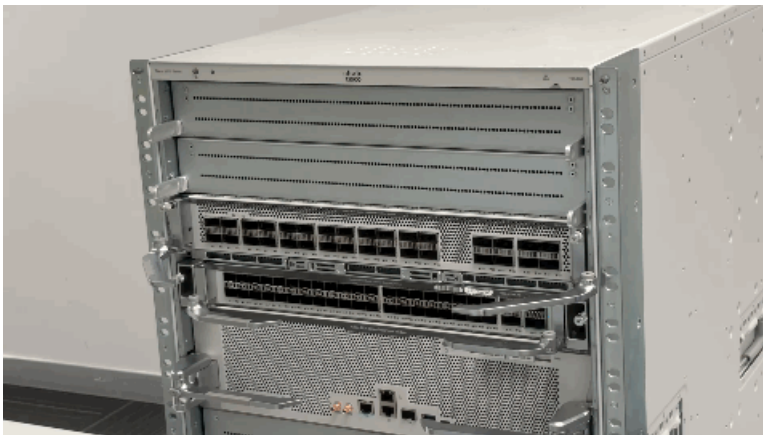
Figure 12: Pivoting the ejector levers outward
