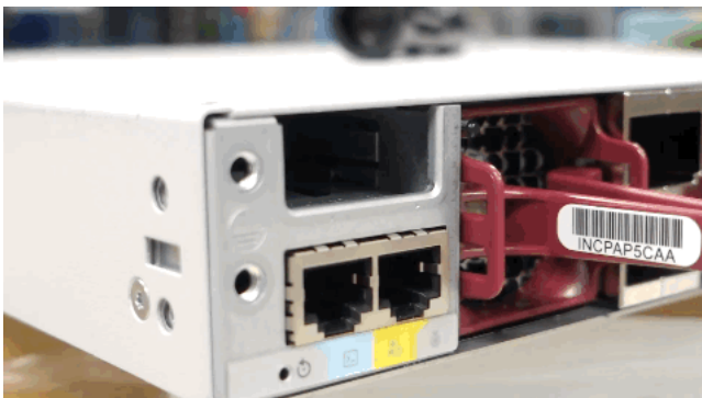
Figure 16: Installing the SSD
