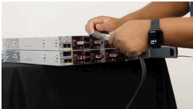
Figure 3: Connecting the StackWise cable in a StackWise port
