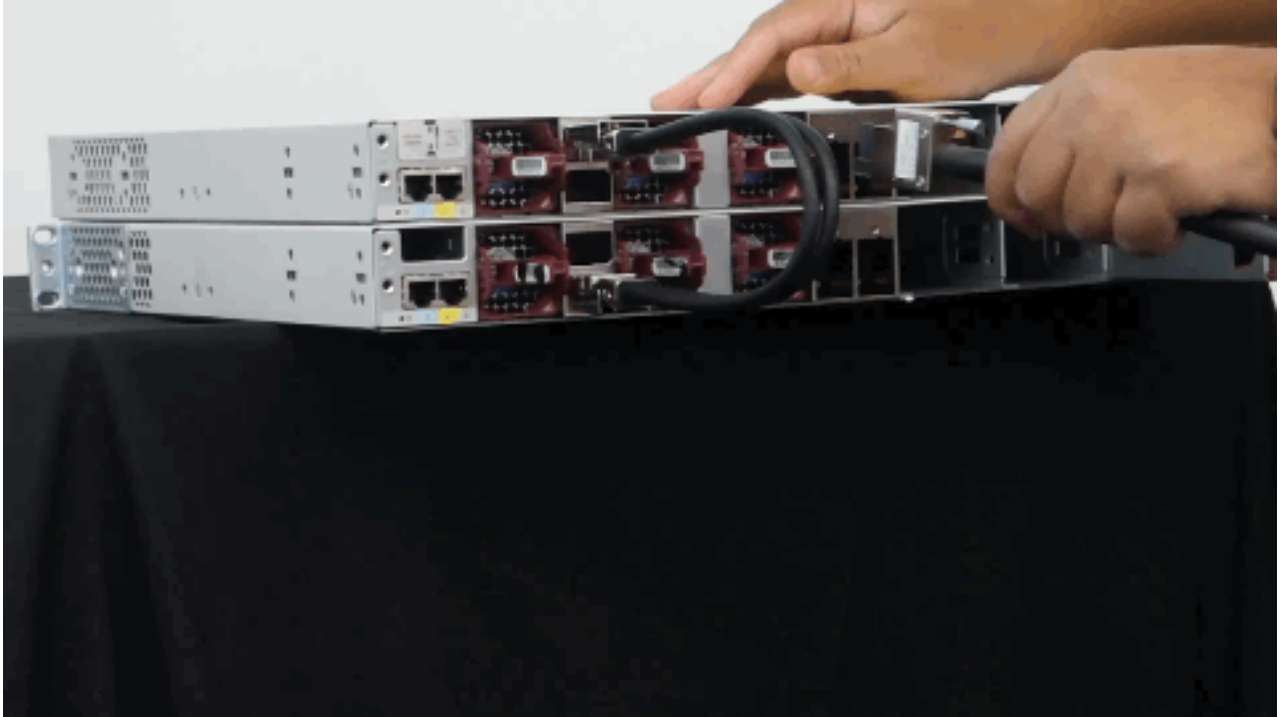
Figure 5: Connecting the StackPower cable
