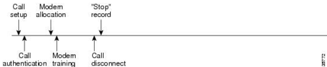
Figure 55: Modem Dial-In Call Setup Sequence With Call Disconnect Occurring Before User Authentication and With Resource Failure Stop Accounting Enabled
