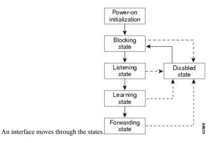
When you power up the device, spanning tree is enabled by default, and every interface in the device, VLAN, or network goes through the blocking state and the transitory states of listening and learning. Spanning tree stabilizes each interface at the forwarding or blocking state.
