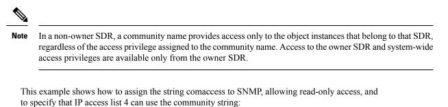
RP/0/RP0/CPU0:router(config) # snmp-server community comaccess ro 4
