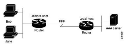
Figure 3: Example Topology for Double Authentication
