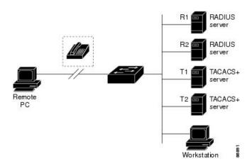
Figure 10: Transitioning from RADIUS to TACACS+ Services
