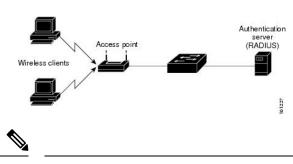
Figure 37: Multiple Host Mode Example
