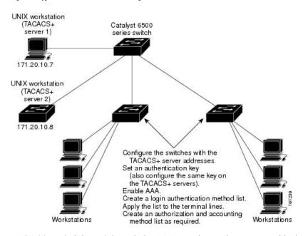
Figure 9: Typical TACACS+ Network Configuration
