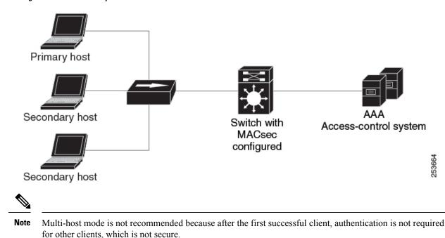
Figure 13: MACsec in Multiple-Host Mode - Unsecured
