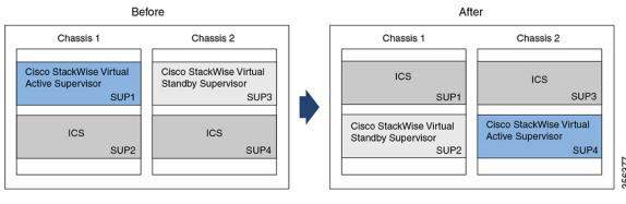
The figure below shows the Quad-Supervisor with RPR with 1 ICS installed in the chassis with the Cisco StackWise Virtual active supervisor before and after ISSU:
