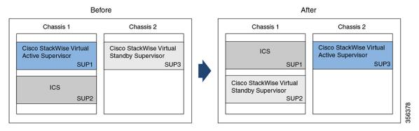
The figure below shows the Quad-Supervisor with RPR with 1 ICS installed in the chassis with the Cisco StackWise Virtual standby supervisor before and after ISSU:
