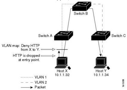
If you do not want HTTP traffic switched from Host X to Host Y, you can configure a VLAN map on Switch A to drop all HTTP traffic from Host X (IP address 10.1.1.32) to Host Y (IP address 10.1.1.34) at Switch A and not bridge it to Switch B.
