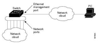
In the above figure, if the Ethernet management port and the network ports are associated with the same routing process, the routes are propagated as follows:
