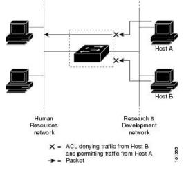
prevent Host B from accessing the same network. Port ACLs can only be applied to Layer 2 interfaces in the
