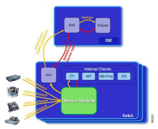
A device with sensor capability gathers endpoint information from network devices using protocols such as Cisco Discovery Protocol, LLDP, and DHCP, subject to statically configured filters, and makes this information available to its registered clients in the context of an access session. An access session represents an endpoint's connection to the network device.
