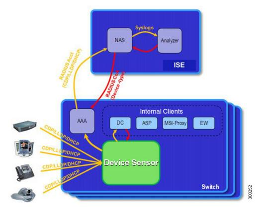
A device with sensor capability gathers endpoint information from network devices using protocols such as Cisco Discovery Protocol, LLDP, DHCPv6, mDNS and DHCP, subject to statically configured filters, and makes this information available to its registered clients in the context of an access session. An access session represents an endpoint's connection to the network device.
