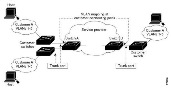
Figure shows a topology where a customer uses the same VLANs in multiple sites on different sides of a service-provider network. You map the customer VLAN IDs to service-provider VLAN IDs for packet travel across the service-provider backbone. The customer VLAN IDs are retrieved at the other side of the service-provider backbone for use in the other customer site. Configure the same set of VLAN mappings at a customer-connected port on each side of the service-provider network.
