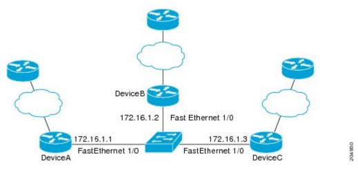
When Fast Ethernet interface 1/0 on DeviceB fails, BFD will no longer detect Device B as a BFD neighbor for DeviceA or for DeviceC. In this example, Fast Ethernet interface 1/0 has been administratively shut down on DeviceB.
