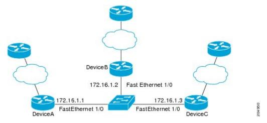
When Fast Ethernet interface 1/0 on DeviceB fails, BFD will no longer detect Device B as a BFD neighbor for DeviceA or for DeviceC. In this example, Fast Ethernet interface 1/0 has been administratively shut down on DeviceB.
