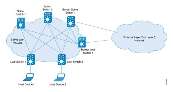
The following image shows a spine-leaf topology with one border leaf switch and one border spine switch connecting the fabric with an external network:
