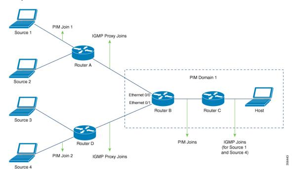
In this method, IGMP proxy is used to enable the user to receive traffic from multiple upstream devices. The following sequence of events occurs:
