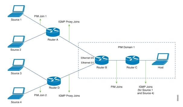
In this method, IGMP proxy is used to enable the user to receive traffic from multiple upstream devices. The following sequence of events occurs:
